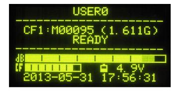
The name of the active profile is shown in the first line. The full profile data will be displayed if the ENTER key is pressed.
