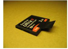
In order to make it easier to remove a CF card from the D500X, a small "handle" can be made with a piece of tape (see the picture).
